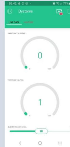
Functional prototype and app. The pen features a pressure sensor measuring how hard you grip the pen and another measuring how hard you write on paper.
