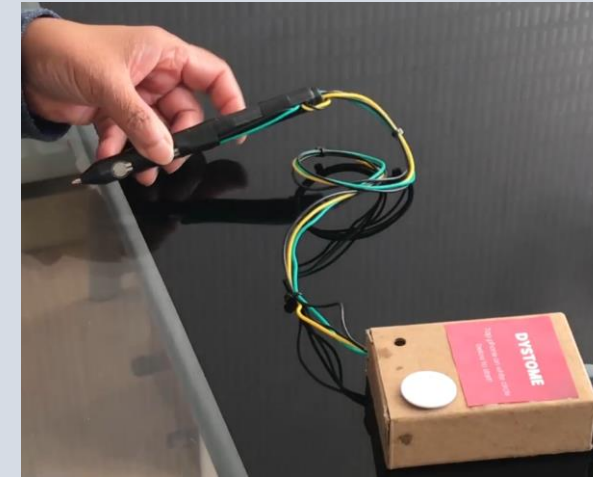
Functional prototype and app. The pen features a pressure sensor measuring how hard you grip the pen and another measuring how hard you write on paper.
